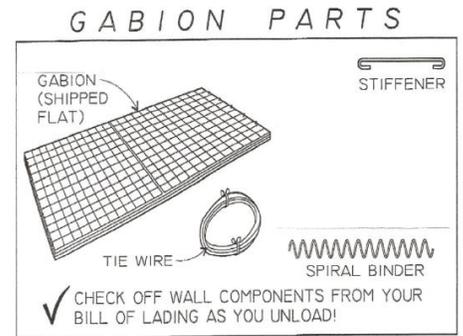
Made in the USA Gabion Baskets are fabricated from precision welded rusty steel wire mesh. Gabions are sold un-assembled in a flat panel kit which can be easily transported and assembled in cells of varying sizes on the job site in minutes. Once erected, they are set into place and filled with decorative rock or rip-rap to form a monolithic, flexible structure.
